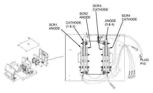
FIGURE F.12 - SCR TEST POINTS.
